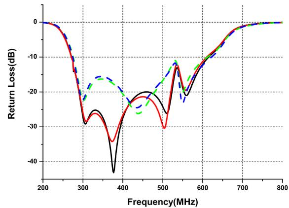
**Fig. 4** A comparison of return loss simulation results for preliminary design (blue and green dotted line) and optimization design (black and red solid line).
